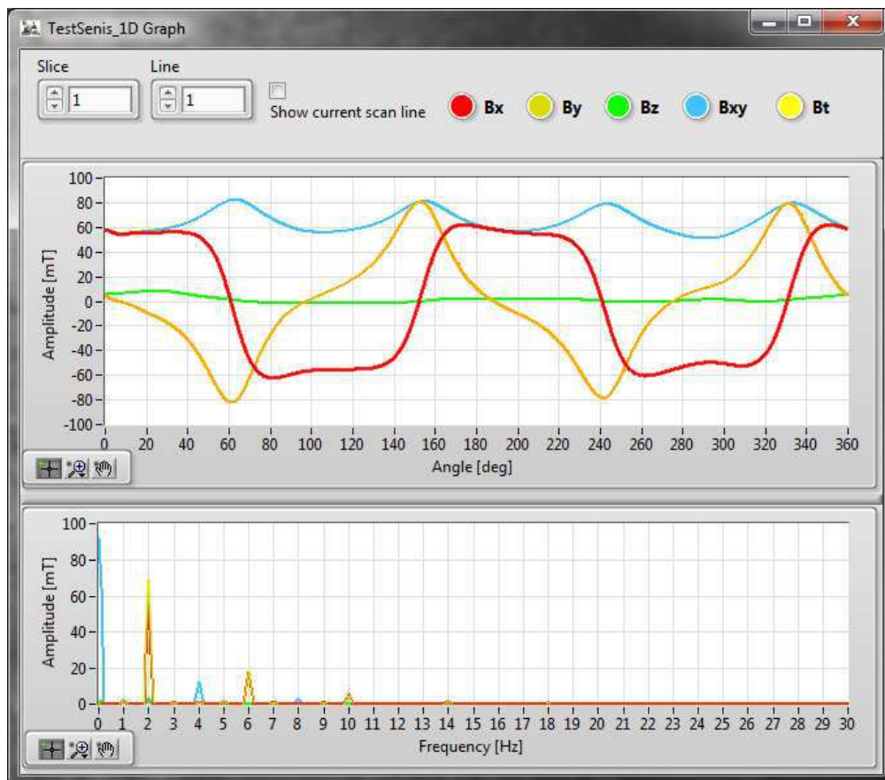
Figure 5: 1D Graph-App: Visualization of all three magnetic field components, B_x , B_y and B_z and B_{xy} , B_{Total} Inclination and Declination, as well as Fourier analysis over different scan slices/lines. The individual component presentation can be switched on and off.
